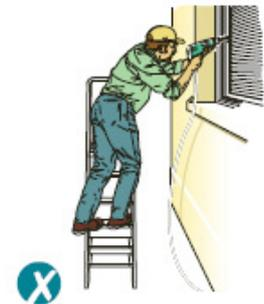
Figure 2a Incorrect - steps side-on to work activity
